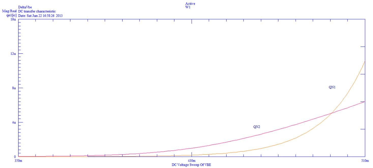
It can be seen from the graph, that there is an intersection of the currents of QN1 and QN2. That is, there are two points where the currents of QN1 and QN2 are equal. One point is at zero  $V_{IN}$ , being zero current in both transistors, the second point being at a “special” equality point.
